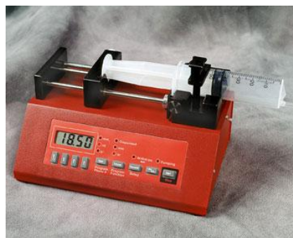
Figure 5. 13: (a) Flash 100 pumping system from LabAlliance ( www.laballiance.com ) (b) Aladdin syringe pump system from WPI ( www.wpi-europe.com )
