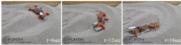
Fig. 18: Experimental results: The robot with compliant joints following a (narrow, 50^\circ ) \Lambda -trench (polychaete mode, f = 1\text{Hz} , \psi = 0^\circ , A = 60^\circ ).
