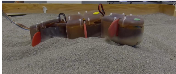
Fig. 2: The Nereis compliant pedundulatory robotic prototype, passively adapting its shape to that of a sand hill.
