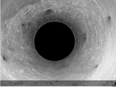
(b) Group B, nozzle machined by ball end mill ( a_p=0.02\text{mm} )
