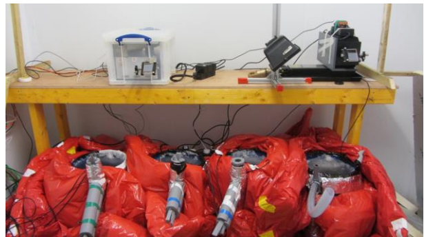
Figure 1. The test setup illustrating both employed hyperspectral systems located above the ice tanks in the cold room.
