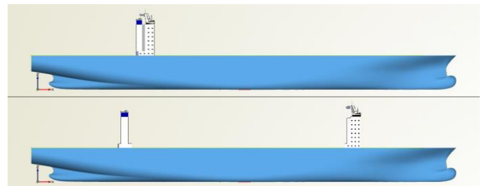
Fig. 5 Alternative superstructure models: Model-1 (above) vs. Model-2 (below)
