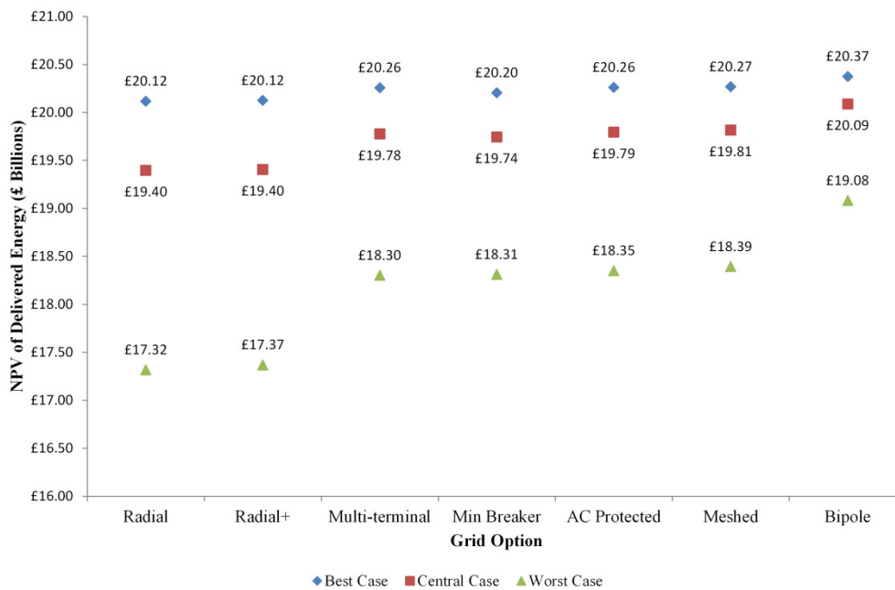
Figure 4.21 - NPV of delivered wind energy for each grid option over project lifetime
