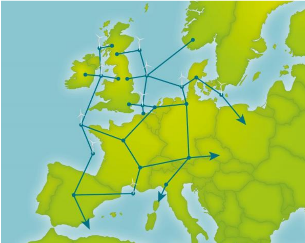
Figure 2.22 - Friends of the Supergrid vision for 2050 HVDC pan European grid [53]
