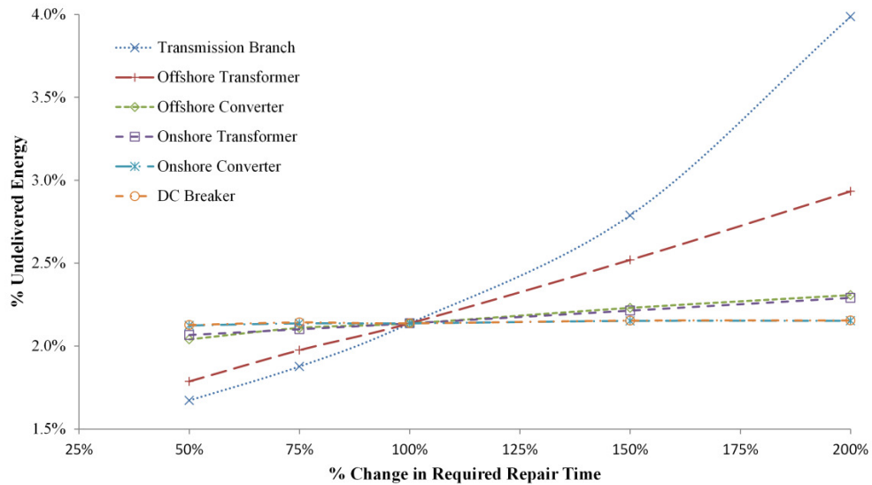
Figure 5.7 - Component sensitivity to repair rate for Dogger Bank bipole grid scenario
