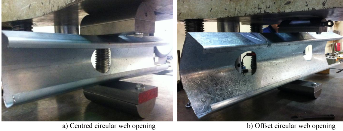
Figure 1: Experimental analysis of cold-formed steel channel sections under ITF loading condition after Uzzaman et al. [13-16]
