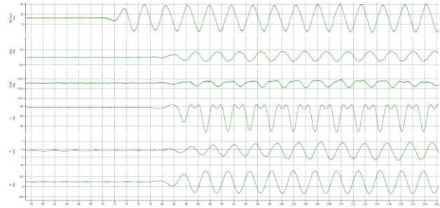
Figure 8 Typical recorded wave and motion data (head waves + SIL) From top: Wave / Pitch / Yaw / Z / Y / X
