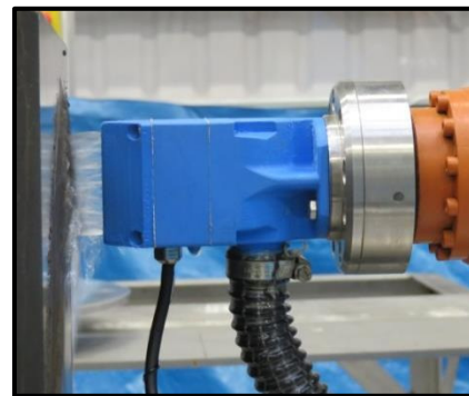
Figure 1 - Example of the type of water jet nozzles used to provide a coupling medium for ultrasonic inspections.
