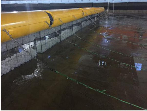
Fig. 6. Three parts of the mooring line.
