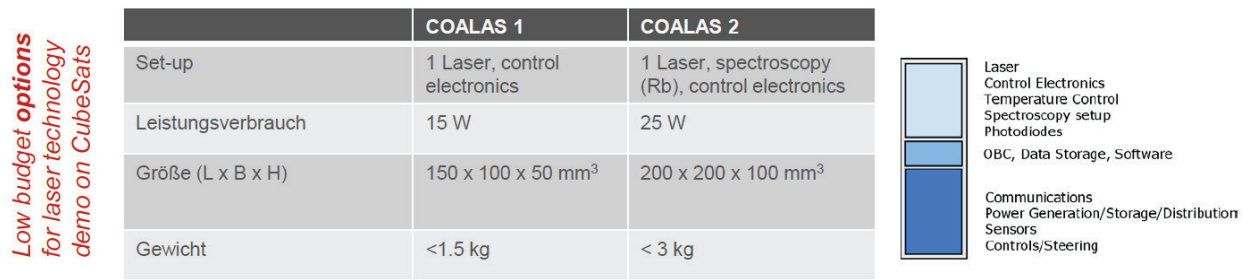
Figure 11. Left: Reduced complexity options for laser system technology tests on nanosatellites: COmpact, AUtonomous LAser payload for Satellite operation (COALAS). Right: Prinipcal architecture of a 3U CubeSat housing COALAS.
