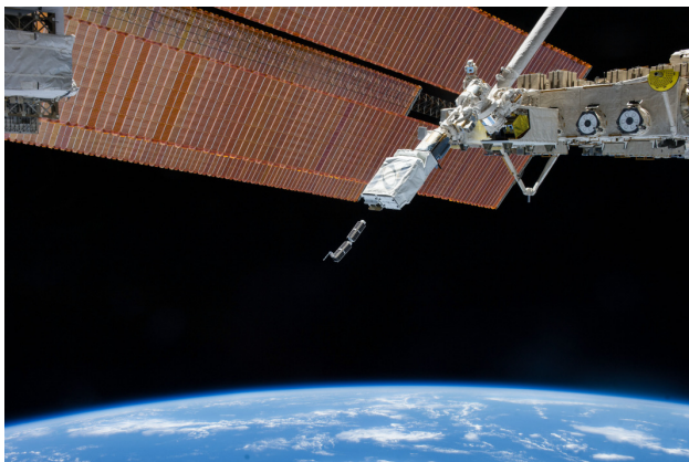
Figure 1. Set of NanoRacks CubeSats Deployed From International Space Station. The Small Satellite Orbital Deployer (SSOD), in the grasp of the Kibo laboratory robotic arm, is photographed by an Expedition 38 crew member on the International Space Station as it deploys a set of NanoRacks 3U CubeSats. This image shows the difference in scale between nanosatellites and the largest man-made structure in space. Credit: NASA
