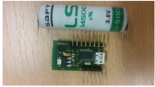
Fig. 4. MSP430+ESP-03 Prototype with Lithium Thionyl Chloride
