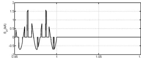
Fig. 6: Waveforms illustrating the capabilities of the proposed switching function based MMC model in capturing detailed behaviour of MMC during dc fault
