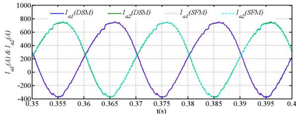
(c) Samples of upper and lower arm currents (phase a, detailed switch superimposed on switching function)
