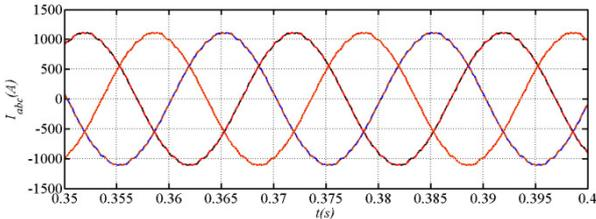
(b) Three-phase load currents (detailed switch superimposed on switching function)
