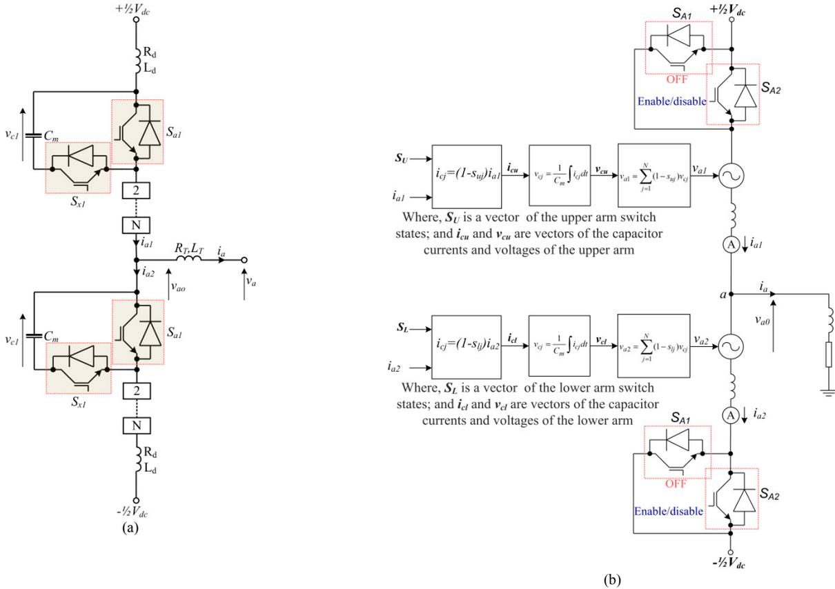
Fig. 1: (a) Generic representation of one-phase-leg of modular multilevel converter, and (b) graphical representation of generic MMC switching function model being proposed
