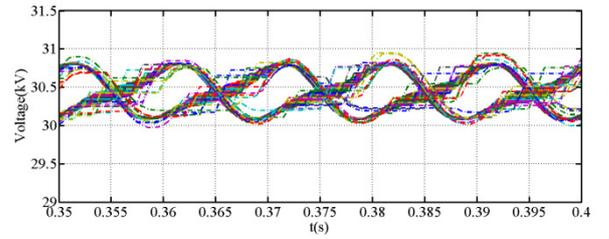
(d) Cell capacitor voltages (phase a, detailed switch superimposed on switching function)
