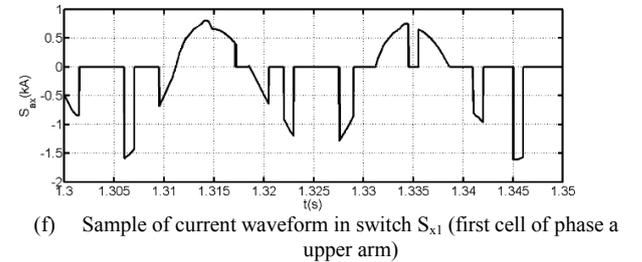
Fig. 5: Waveforms illustrating the capabilities of the proposed switching function based MMC model in capturing detailed behaviour of MMC during normal operation
