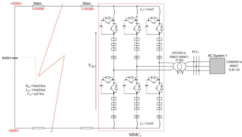
Fig. 4: Illustrate test system used to validate the proposed MMC switching function model
