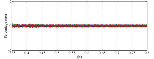
(e) Percentage error in the three-phase output currents (detailed switch versus switching function)
