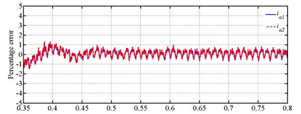
(f) Percentage error in the arm upper and lower arm currents (detailed switch versus switching function)
