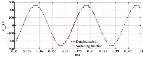
(a) Output phase voltage ( $V_{ab}$ , detailed switch superimposed on switching function)
