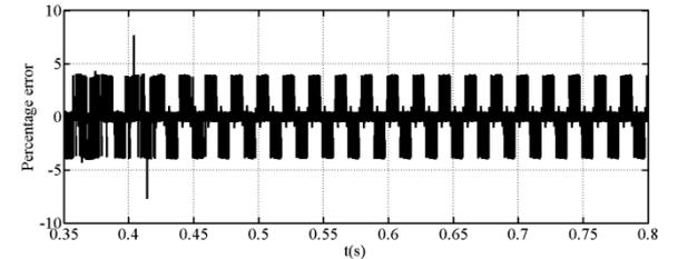
(g) Percentage error in the phase output voltage (detailed switch versus switching function)
