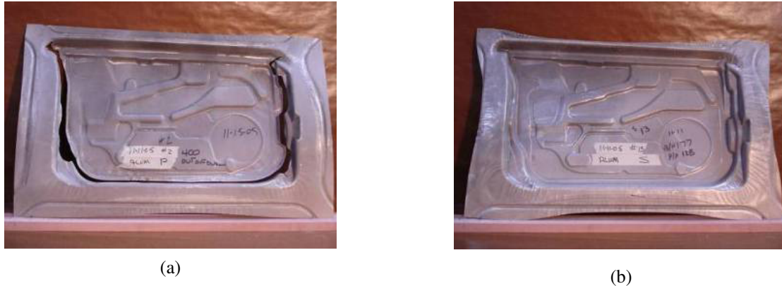
Fig.4. Inner door a) poor formability at room temperature lead to failure. b) Warm forming of the inner door. [15].
