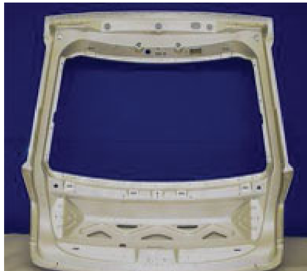
Fig.10. Hot forming of aluminum alloy Chevrolet Malibu Maxx lift gate [16].
