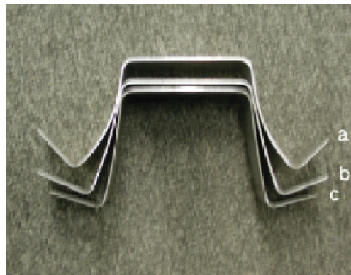
Fig.5. Effect of Springback on A5182 formed at a) room temperature b) 250°C and c) formed steel at room temperature .[14]
