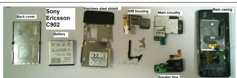
Fig. 6 Photo of the disassembled Sony Ericsson C902
