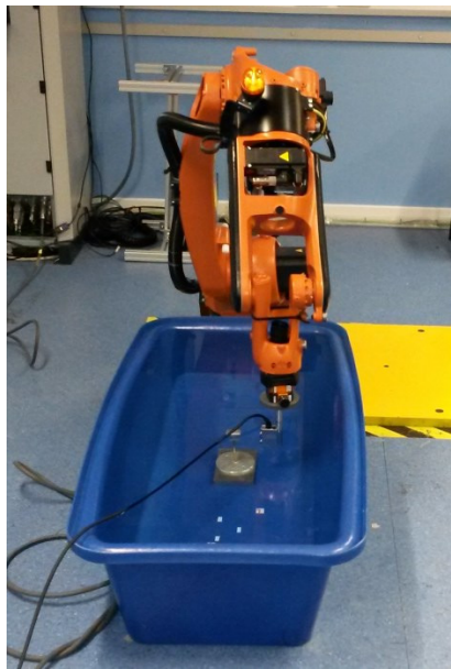
239 Fig. 5: Experimental setup, showing the submerged sample, with the probe face fully 240 submerged.
