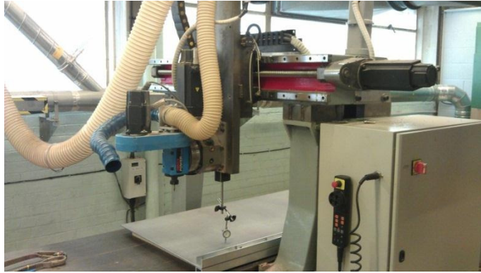
Figure 2: Checking the flatness of the plates.
