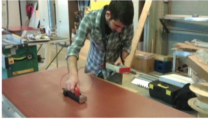
Figure 9: Measurement of the roughness of F0037 using a TQC Hull Roughness Gauge.
