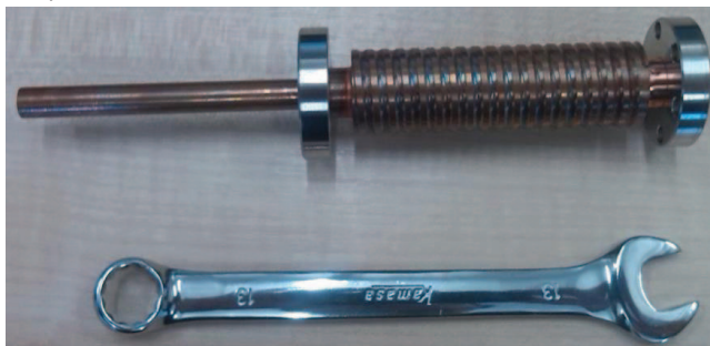
Fig. 4 A photo of water-cooled electron beam dump.
