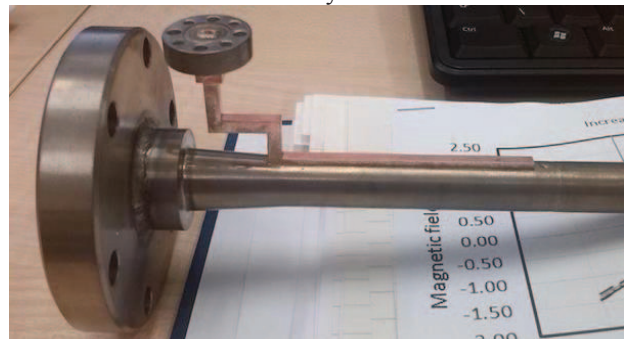
Fig. 3 A photo of the upgarded input coupler.
