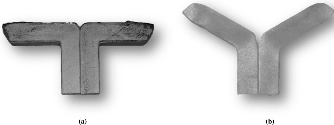
Figure 5: I-ECAPed billets halfway processed (a) \phi=90^\circ and (b) \phi=120^\circ
