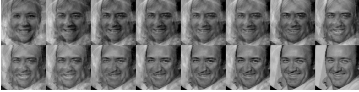
Figure 2.13: A step by step application of the weighted eigenvectors being added to the mean face in order to reform the original image of Kevin Spacey.
