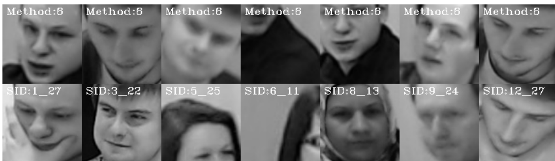
Figure 4.30: Example output from the system where the ensemble method is used with nearest neighbourhood k = 4 ; using the single pass approach on lecture 12. The top row of the figure represents the face images captured at the lecture and the bottom row shows the student to which they were matched.
