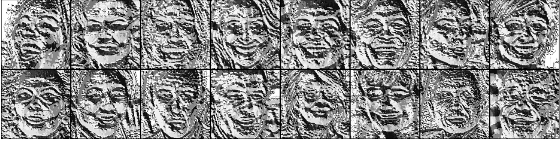
Figure 2.19: An encoding of the baseline LFW data set using the LBP technique.
