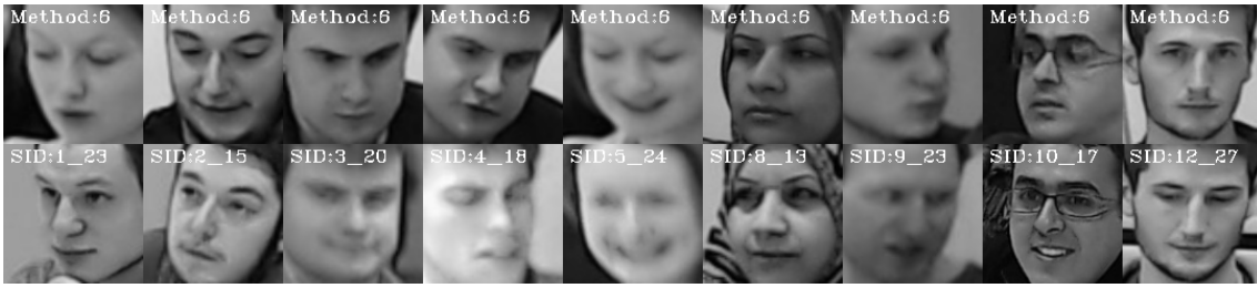
Figure 4.36: Example output from the system where the ensemble method is used with nearest neighbour k = 4 ; using the single pass approach on lecture 13. The top row of the figure represents the face images captured at the lecture and the bottom row shows the student to which they were matched.
