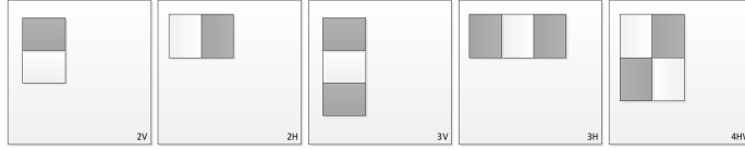
Figure 2.4: Three distinct types of Haar-like feature are defined and are identified by the number of adjacent rectangles they contain (two, three or four) and the relative positions of their rectangles. Each feature is available in both horizontal and vertical forms. Each distinctive area is a template used to compute contrast information when computed over the image space.
