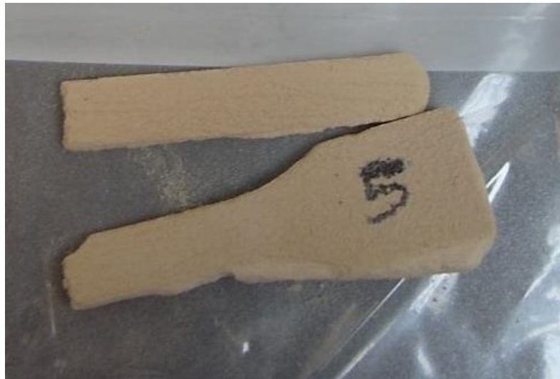
Figure 17. PEEK 450PF laser sintered sample manufactured with build parameters corresponding to EMR = 1 .
