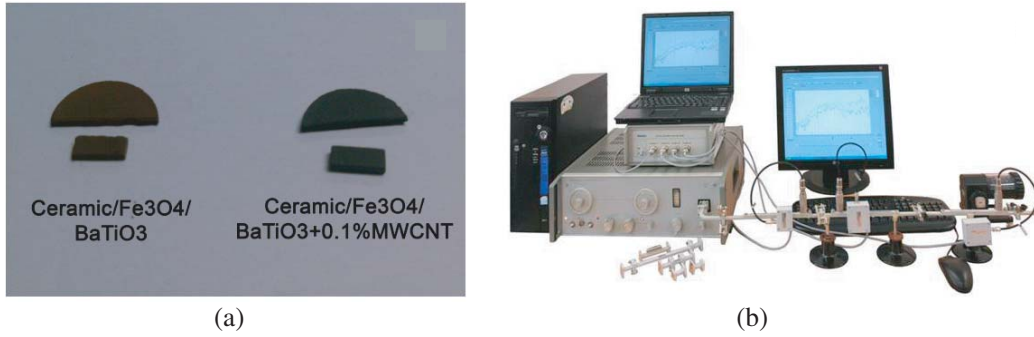
Figure 5. (a) General view of prepared composites without MWCNTs (left) and with 0.1 wt.% of MWCNTs (right); (b) Scalar network analyser ELMIKA R2-408R used for Ka-band measurements.
