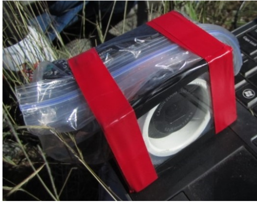
Figure 8-6. Camera sensor sealed in dust-proof protective casing.
