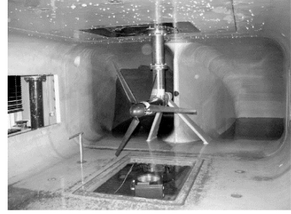
Figure 3 Experimental setup of 1/20th scale model TST in a cavitation tunnel for cases 1a and 1b [8]
