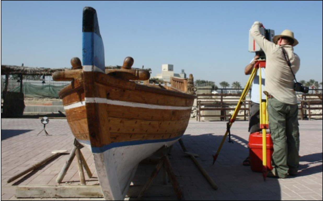
Figure 2: Setting up the scanner and tripod alongside the banūsh, the smallest of the vessels scanned.
