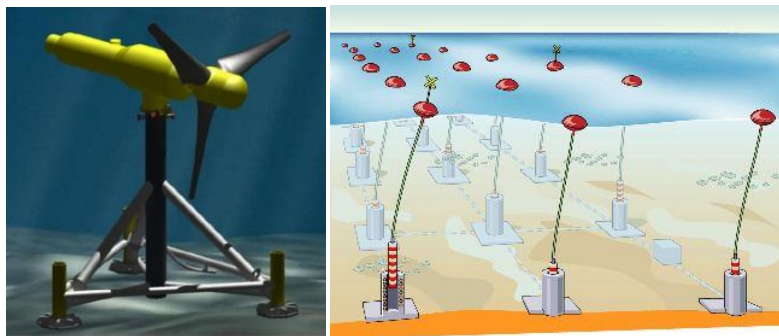
Figure 1. ( left ) Alstom/TGL 1-MW turbine (image source: [8]) and ( right ) Uppsala University wave power plant (image source and copyright: Karl Astrand and Division for Electricity, Uppsala University; [9]).
