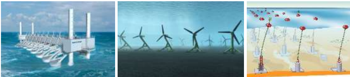
Figure 1: Artist’s impressions of MRE arrays: (left) Wave Star wave energy converter, (middle) ScottishPower Renewables Sound of Islay 10MW tidal turbine array, (right) Uppsala University wave power plant
