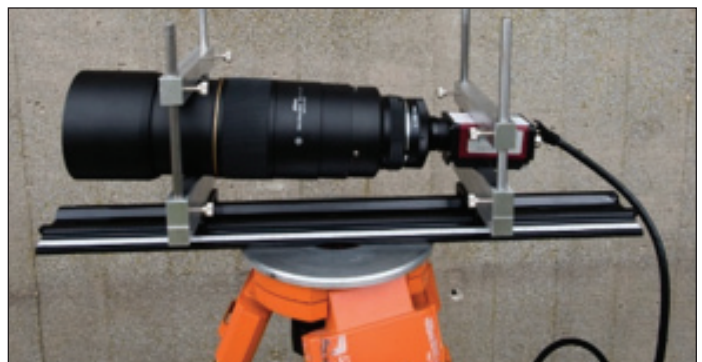
Figure 1: Mounting configuration of the camera and 300 mm lens
