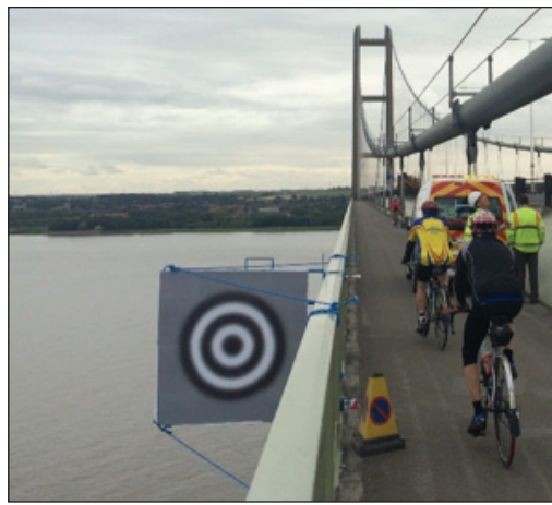
(b) Custom-made target installed at mid-span
