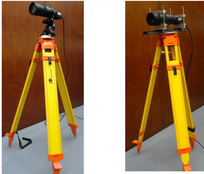
Figure 6. Lens mounting, (left) old approach, (right) new approach
