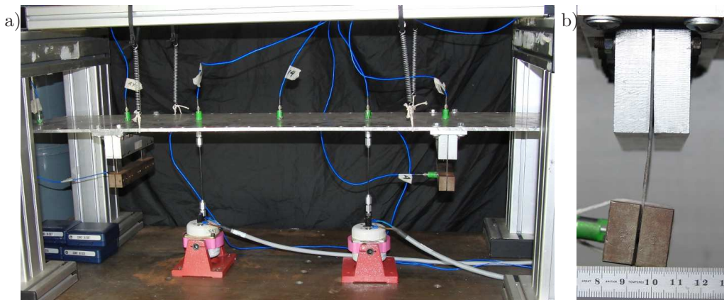
Figure 10: Test structure representing the configuration of an aircraft wing having two underwing stores supported by pylons. a) General view of the experimental setup. b) Close up of the nonlinear connection.
