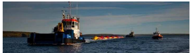
Fig. 1 The use of inexpensive, readily available, multipurpose workboats is fundamental to Pelamis Wave Power's O&M strategy.
