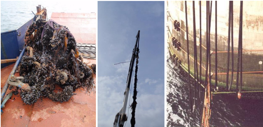
Figure 16: ( left ) Recovered nylon mooring rope used during the first deployment of SWMTF. Considerable bio-fouling in the form of mussel growth and kelp can be observed, ( middle ) removal of fouling using the on-board crane. ( right ) An example of bio-fouling prevention; polyurethane coated polyester riser protection net after four years of service on the Heidrun TLP.
