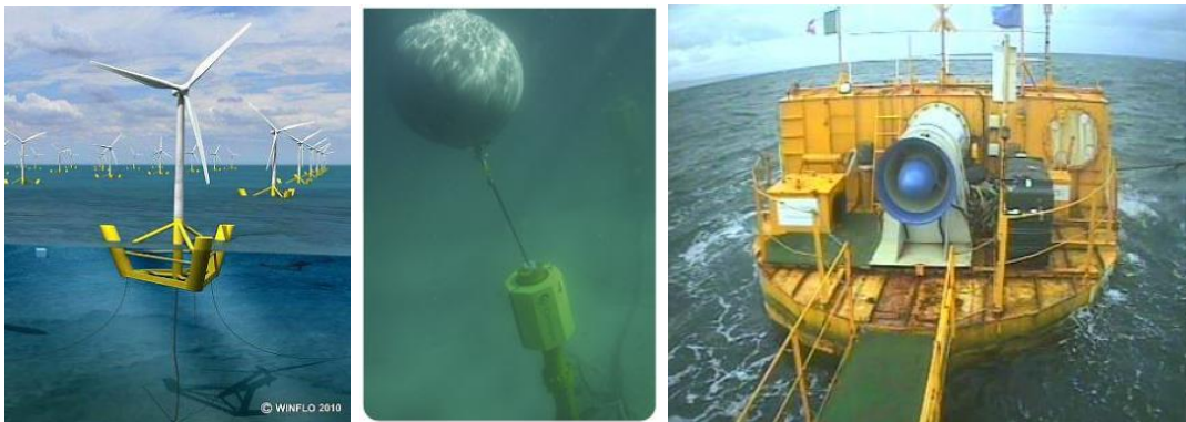
Figure 18: MRE device examples which utilise synthetic mooring ropes; (from left) WinFlo concept (source: WinFlo), CETO wave energy device (source: Carnegie Wave Energy) and CORES oscillating water column [50]. Images accessed online: 21/09/2013
