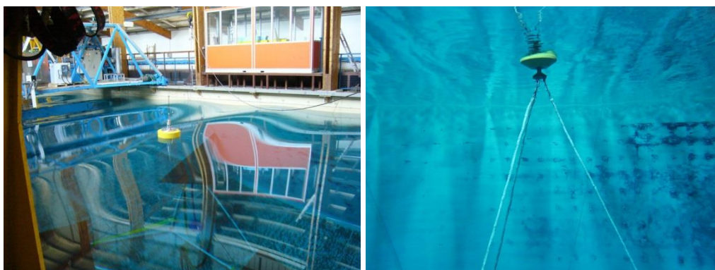
Figure 17: (left) 1:5 scale model of the SWMTF tested in the salt water basin at IFREMER, (right) underwater view of small-scale lines with representative bio-fouling [48].
