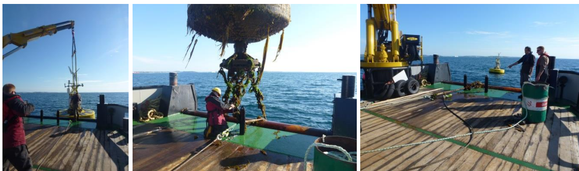
Figure 15: Example operation showing recovery of one SWMTF mooring rope using on-board crane and winch of the work boat
