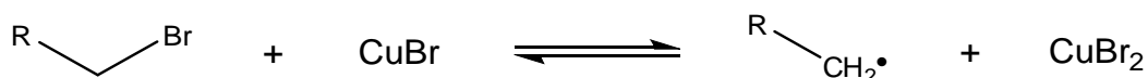
Figure 4.3. ATRP initiation/deinitiation through equilibrium reaction of copper bromide with alkyl bromide and alkyl radical sites
