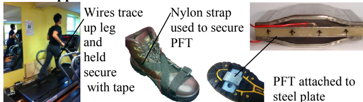
Figure 5. Testing of PFT in a shoe using a treadmill. PFT retrofitted into shoe with extra steel plate and held in place with nylon strap.
