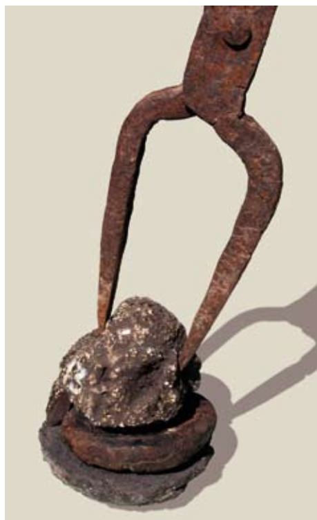
Fig. 4 Combined crucible body and lid fragment, steel ingot and traditional steel-maker's tongs (author's collection)
