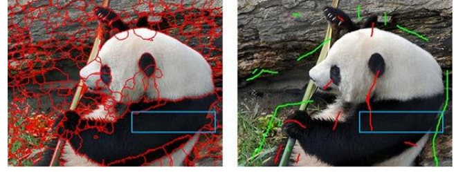
Fig. 3. Illustration of processing the conflicting superpixel between foreground scribbles and background scribbles. (a) The image of superpixels; (b) the user scribbled image.
