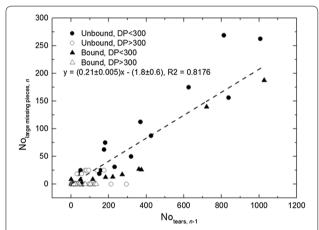
**Fig. 8** Accumulation of large missing pieces in the challenge number *n*, as a function of the number of all tears in the preceding challenge (*n*-1), both per 100 sheets, for bound and unbound volumes. The *regression line* is drawn using all data points
