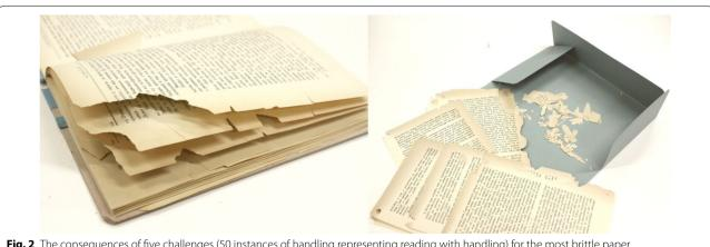
Fig. 2 The consequences of five challenges (50 instances of handling representing reading with handling) for the most brittle paper
