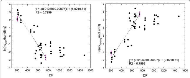
**Fig. 9** *Left* accumulation of large missing pieces (text missing) per handling, i.e. leafing through the entire document once as if reading/searching for information, of paper (per 100 sheets) depending on the DP of paper. *Right* number of handlings until such paper develops one large missing piece per 100 sheets, depending on their DP. *LMP* large missing pieces (i.e. a piece with text missing)
