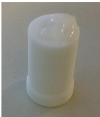
Figure 3.12: Gel Stuck on RAFT Absorber. Removal of the absorber from the gel before 15 minutes repeatedly resulted in the gel remaining attached to the absorber resulting in the continued absorption of liquid from the gel.
