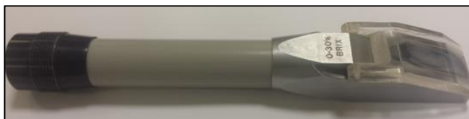
Figure 30: A B+S handheld refractometer (0 to 30 % Brix) with 0.2% graduations.
