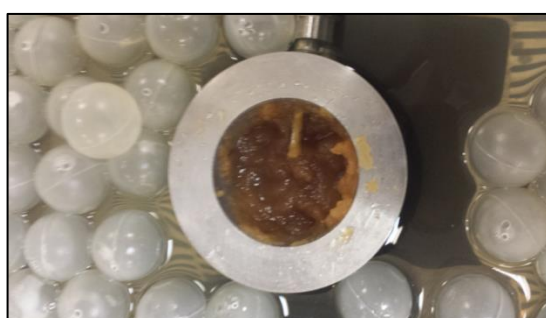
Figure 33: Picture from the top of the apple puree in a Cygnus UVM1 Ultrasonic Velocity Meter (UVM) cell measurement immersed in the water bath
