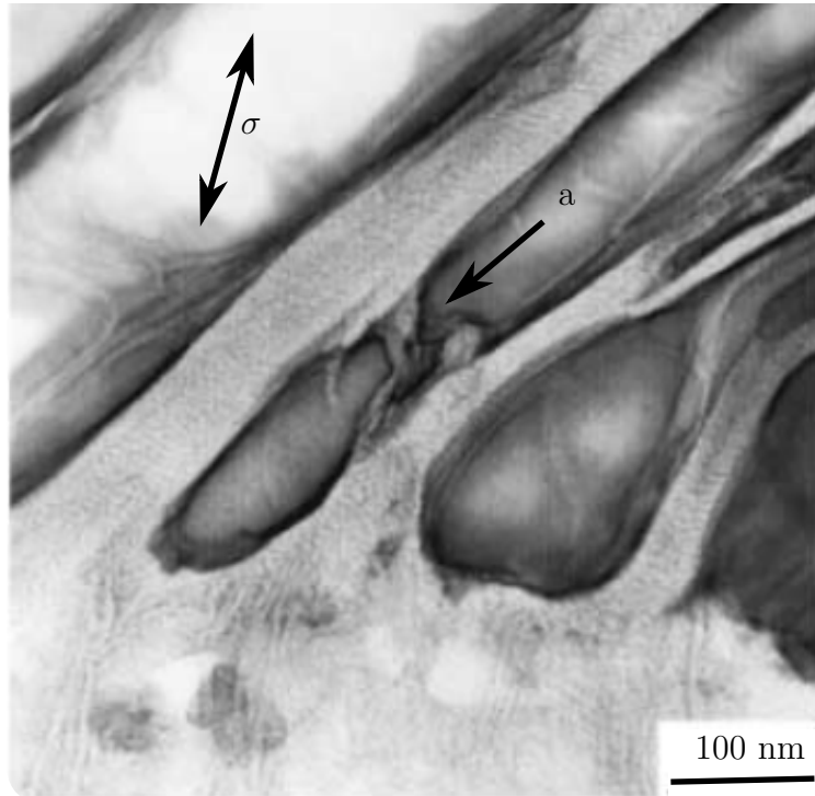
Figure 1.16: Transmission electron micrograph of a section through the fracture surface of a polyethylene-butene copolymer. The direction of the applied stress \sigma is indicated, and (a) indicates a cross tie fibril. Image reproduced from [89]
