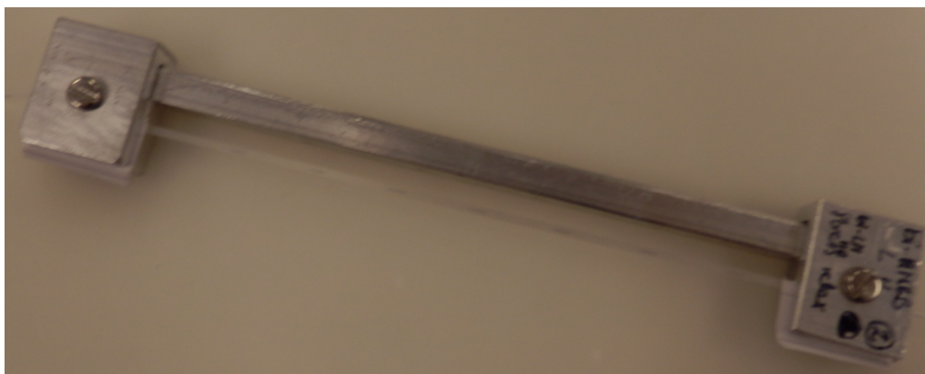
Figure 2.1: Harness used to keep specimens under strain after taking out of the Instron
