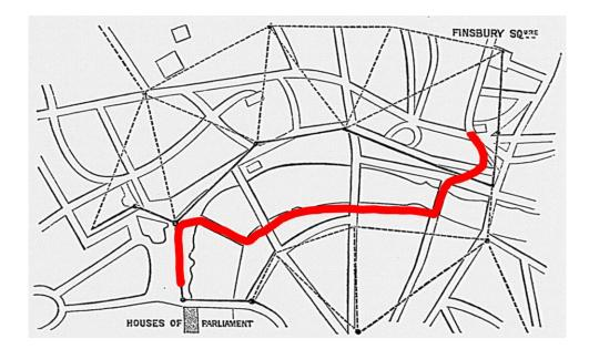
Figure 4.2. Waterlow's private network (1857) from London Wall to Parliament Street, via the Southwark and Hungerford bridges: an approximate path (thick red line) has been overlayed on a map of London published in an article titled 'The nervous system of the metropolis' on 2 March 1861 in the magazine *Once A Week*. The other plain and dotted lines represent the intended route of the future UPTC network (see Figure 4.5.).
