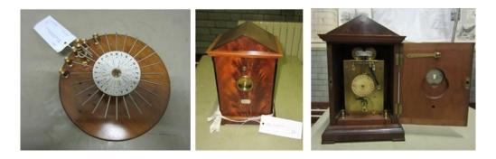
Figure 4.1. Charles Wheatstone's original 1840 dial instrument (Patent No. 8345), based on the stepby-step technology: the 'Communicator' on the left, and the 'Indicator' on the right (battery not shown). See Appendix 4 for a full history of the step-by-step technology and the ABC instrument. Photographed at Blythe House in September 2013, and reproduced with the kind permission of the Science Museum London.
