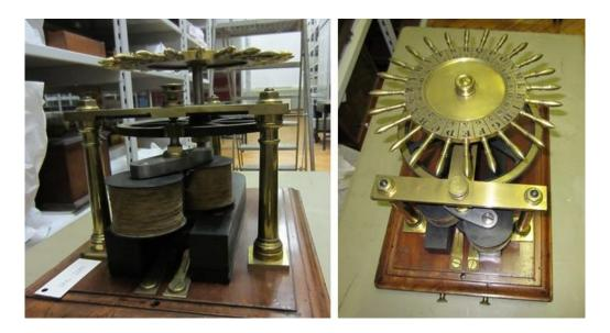
Figure A 4.3. Magneto-Electric ABC Instrument, 1840 specification. Photographed at Blythe House in September 2013, and reproduced with the kind permission of the Science Museum.
