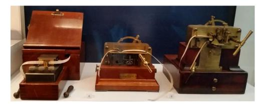
Figure 5.3. Picture of a Wheatstone Automatic Instrument. It consisted of three distinct devices: the perforator with the dispenser of paper behind it (left), the transmitter (centre) and the receiver (right). Photograph taken at the Porthcurno Telegraph Museum in Cornwall and reproduced here with their kind permission.
