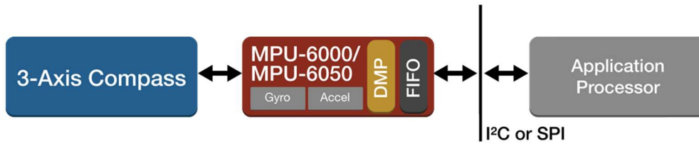
Figure 3.10: MPU-6050 system diagram (InvenSense, 2013)
