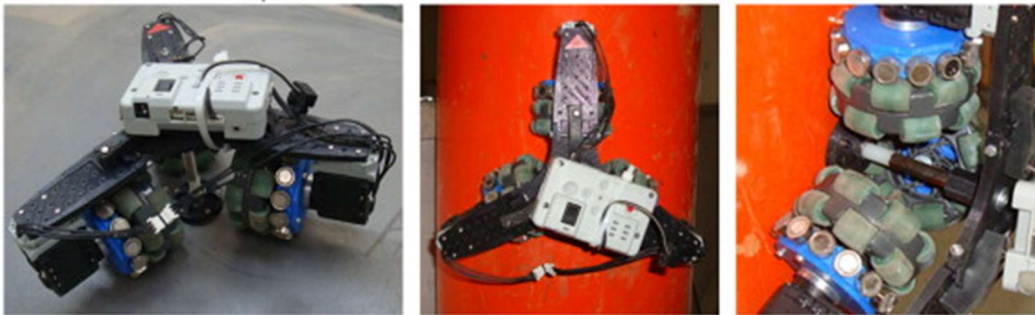
Figure 1.4: Omniclimber, magnetic wheeled climbing robot (Tavakoli et al 2013)
