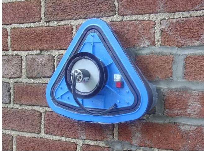
Figure 1.3: City-Climber using vortex force for adhesion (Xiao et al., 2005)
