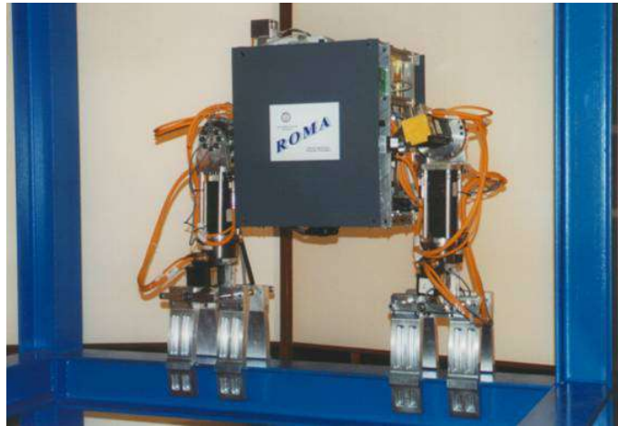
Figure 1.6: ROMA robot climbing a beam-based structure
