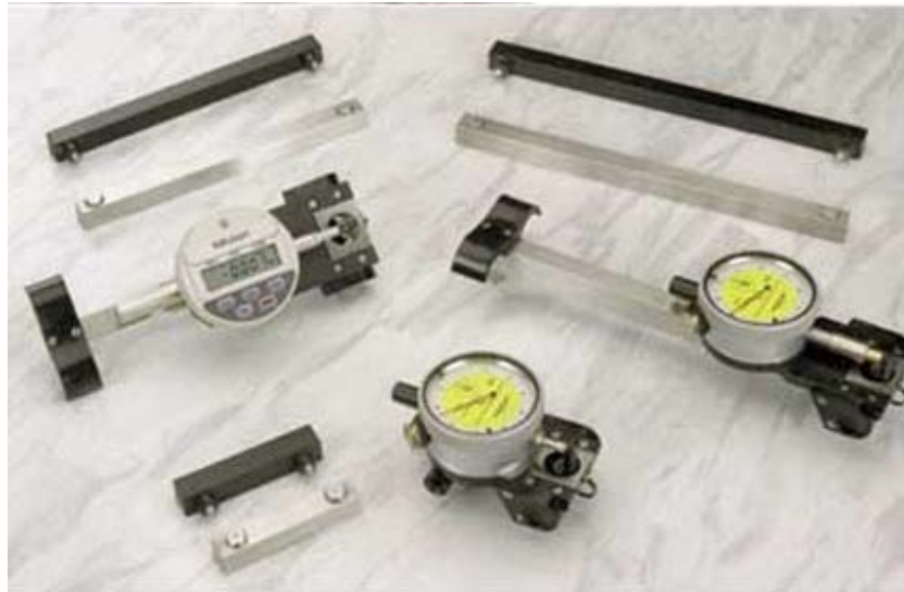
Figure 3.6 DEMEC gauge measurement
