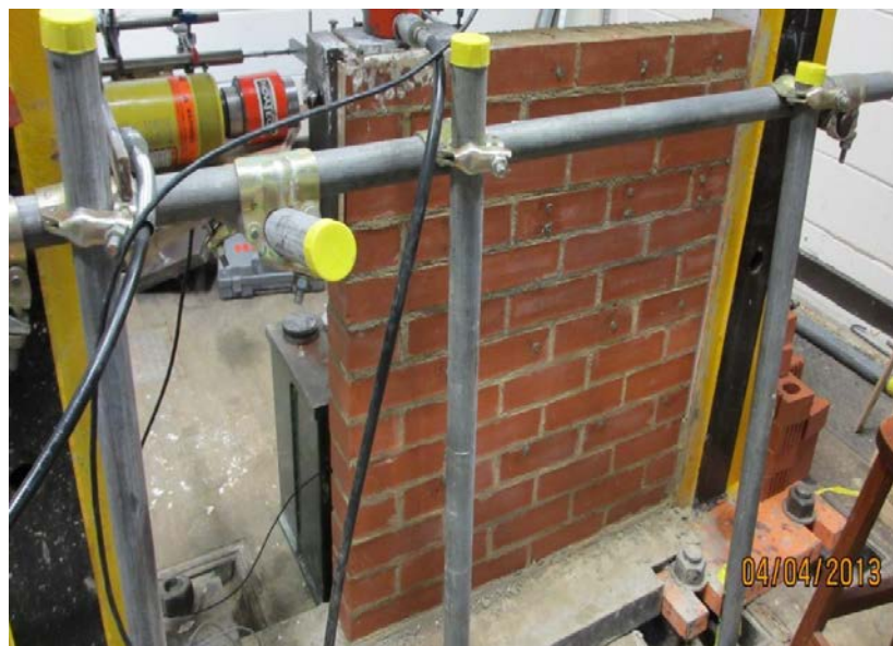
Figure 3.7 Test rig of single-leaf wall on the front side
