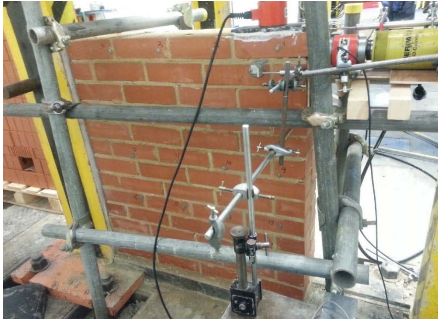
Figure 3.10 Test rig of double-leaf wall on the front side
