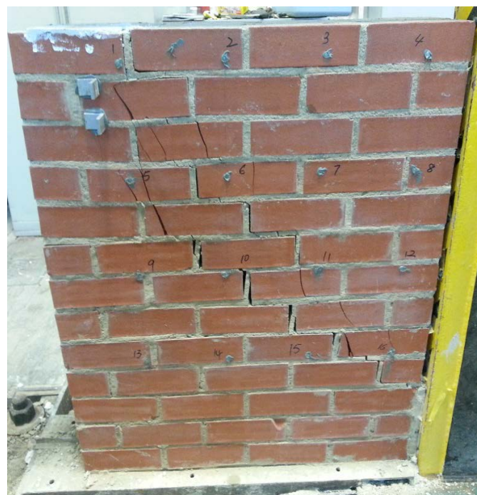
Figure 4.7 Failure pattern of double leaf wall W5 on the loaded leaf
