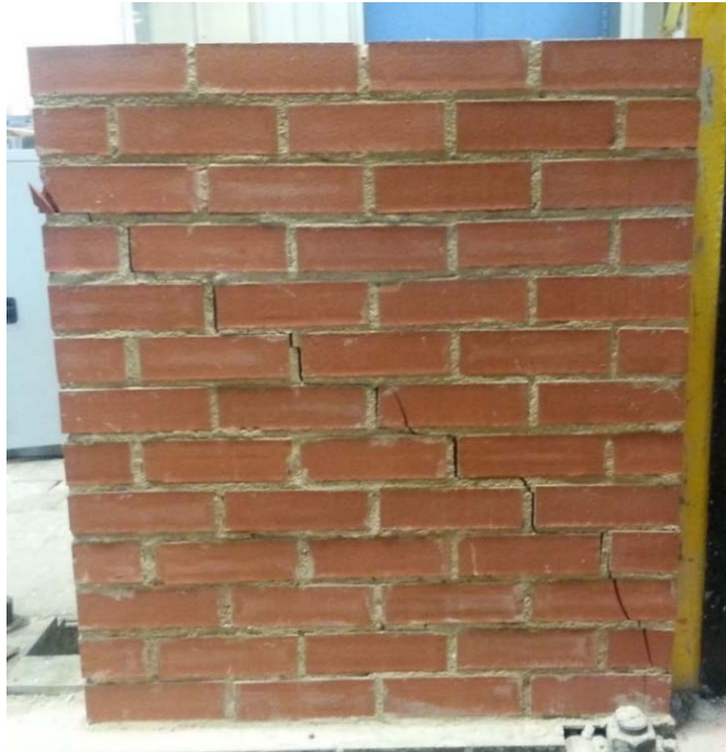
Figure 4.6 Failure pattern of double-leaf wall W4 on the unloaded leaf
