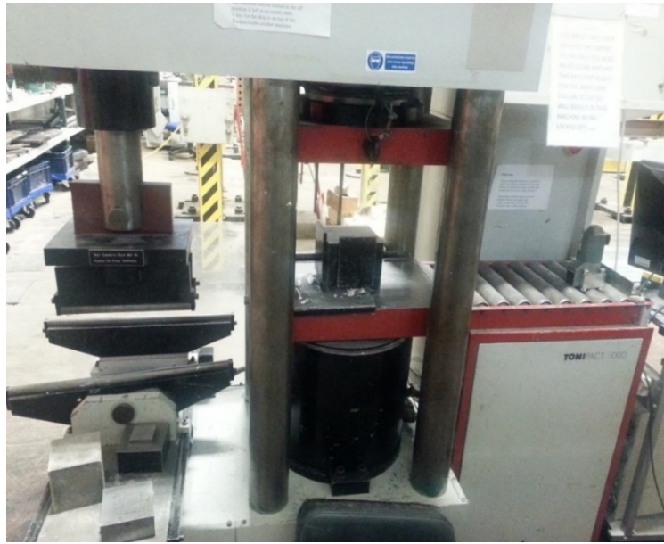
Figure 3.2 TONI PACK for compression test
