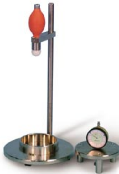
Figure 3.4 Dropping ball apparatus
