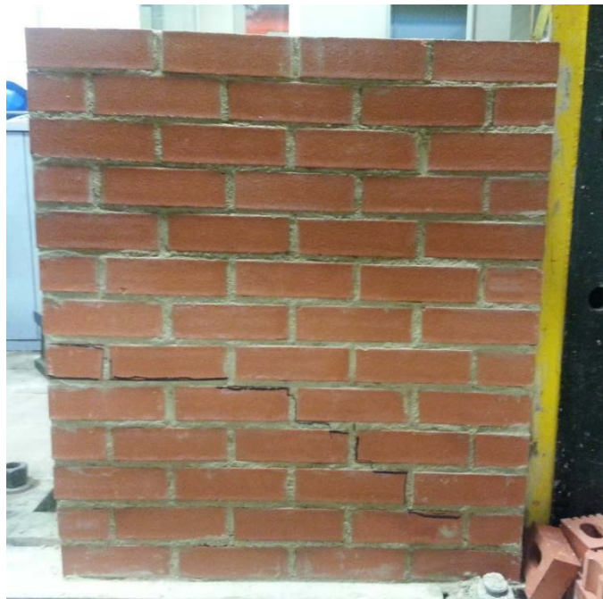
Figure 4.10 Failure pattern of double-leaf wall W7 on the back side
