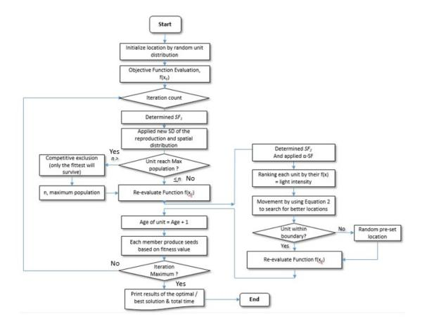
Figure 3.8: The flow-chart of HIWFO-SF algorithm.
