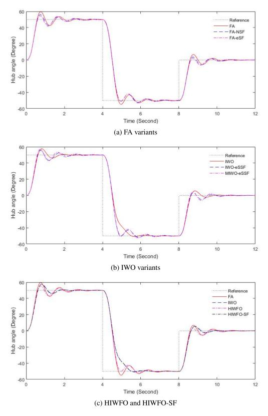
Figure 6.19: Hub-angle response of the single-link flexible manipulator
