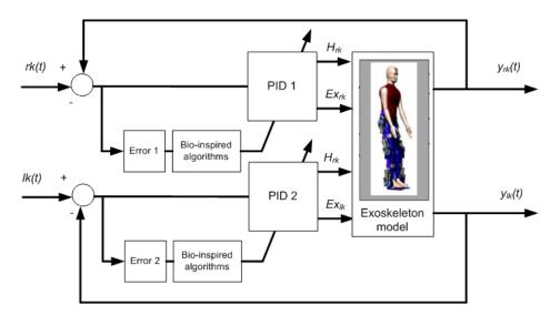
Figure 6.28: Lower limb exoskeleton with PID control
