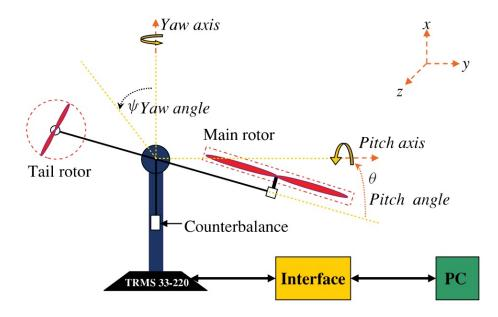
Figure 6.1: Schematic diagram of TRS
