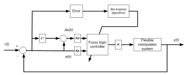
Figure 6.14: The block diagram of PD-fuzzy logic control for single-link flexible manipulator
