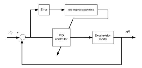
Figure 6.21: PID-based bio-inspired control mechanism of exoskeleton system
