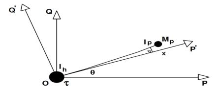
Figure 6.13: Single-link flexible manipulator representation (Azad, 1994)
