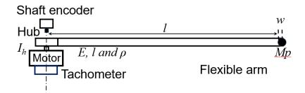
Figure 6.12: Schematic diagram of flexible manipulator system
