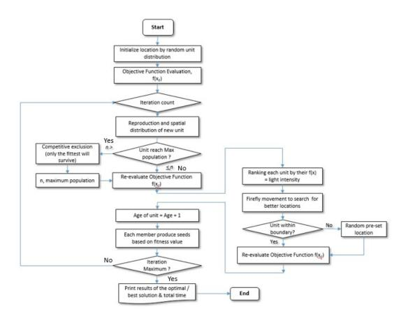
Figure 3.7: The flow-chart of HIWFO algorithm.
