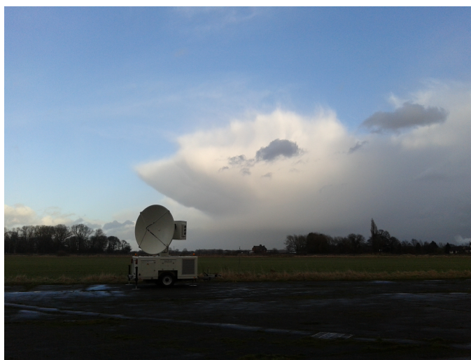
FIGURE 3.1: The modified Meteor 50DX operated by NCAS deployed at the Burn testing site, 30-01-2013. Notice the absence of a radome due to the oversized parabolic antenna fitted to the radar.
