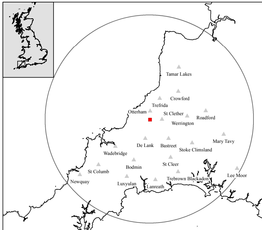
FIGURE 3.6: Location of the rain gauges telemetered by the Environment Agency (grey triangles). Davidstow radar site is shown with red square and 50 km range ring is shown for scale.
