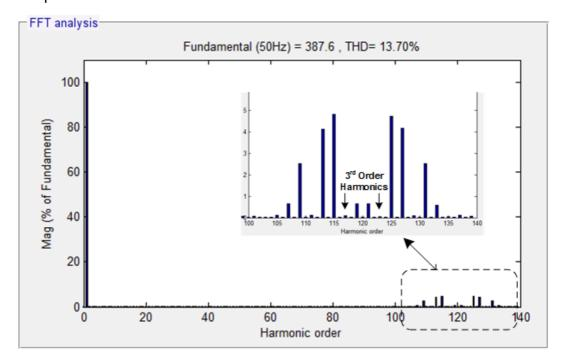
Figure 3.15: Line Voltage Spectrum & THD for PS-PWM at  $m_f$  =15
