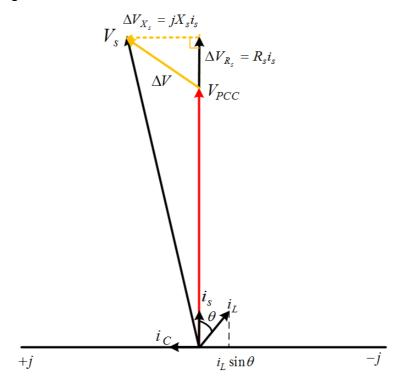
Figure 5.4: Phasor Diagram showing Unity Power Factor Operation
