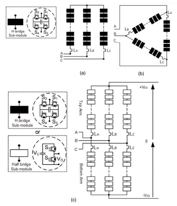
Figure 1.9: Power Circuit Configuration (a) Single Star Bridge Cells (b) Single Delta Bridge Cells (c) Double Star Chopper/Bridge Cells
