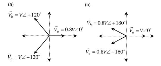
Figure 4.8: (a) Single phase grid fault – Type B (b) Phase to phase grid fault -Type C
