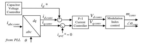
Figure 7.6: Block Diagram for Pre-Charge Control
