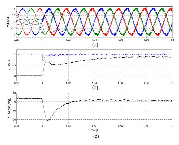
Figure 5.16: (a) Three Phase Voltage and Current, (b) Voltage Magnitude and Current Magnitude, (c) Power Factor Angle
