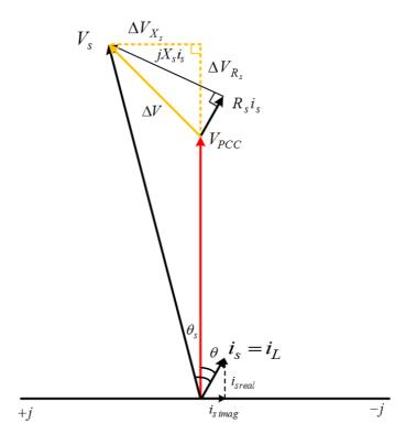
Figure 5.2: Phasor Diagram between Grid Side and PCC
