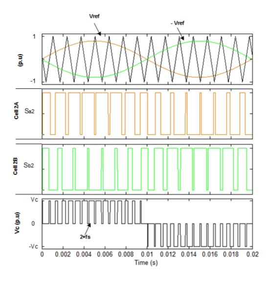
Figure 3.4: Unipolar Switching of Unit Cells
