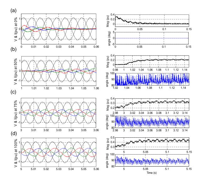
Figure 7.11: Voltage, Current and Converter Angle, (a) Zero compensation, (b) 50% compensation, (c) 75% compensation, (d) Full compensation
