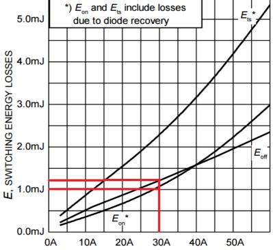
Figure 2.4:Characteristics of the IGBT current and switching energy losses [144].
