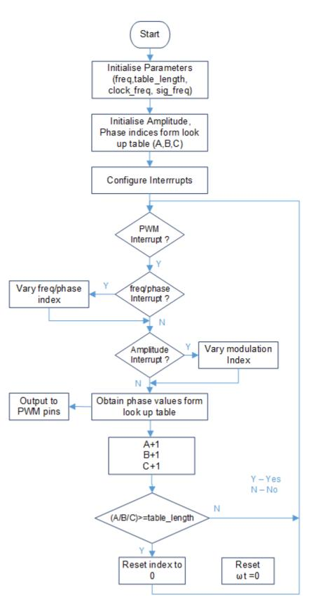
Figure 4.15: Voltage Generation Program Flow Chart
