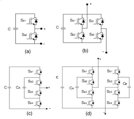
Figure 2.1: MMC Sub-modules (a) Half-Bridge (b) H-bridge (c) FC Halfbridge (d) FC H-bridge
