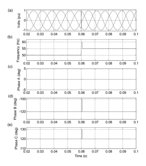
Figure 4.7: EO-PLL Under Balanced Voltage Conditions
