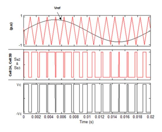
Figure 3.2: Bipolar Switching of Unit Cells
