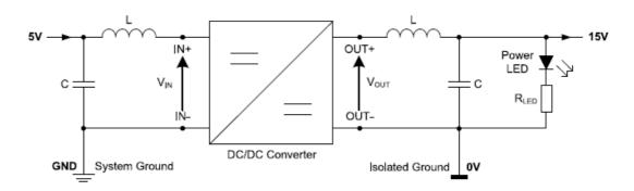
Figure 6.14: +15V Switch Mode Power Supply
