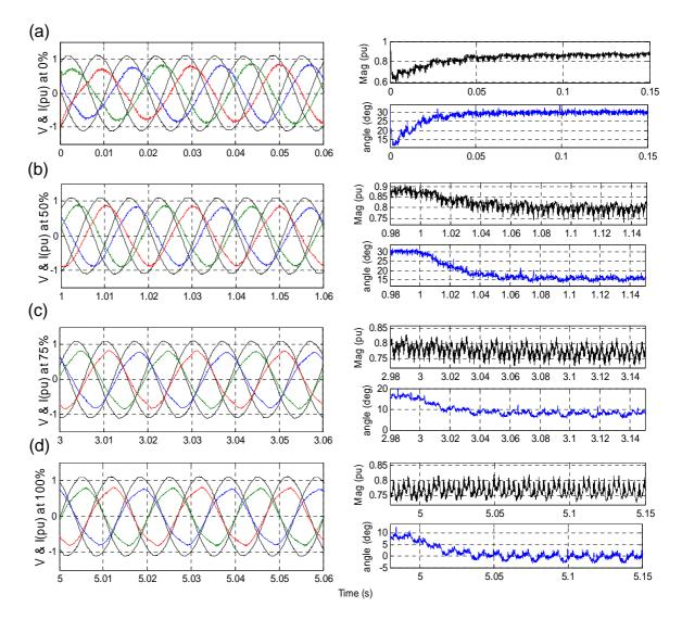
Figure 7.10: Voltage, Current and Power Factor Angle, (a) Zero compensation, (b) 50% compensation, (c) 75% compensation, (d) Full compensation
