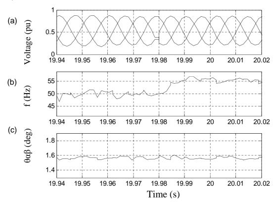
Figure 4.18:Experimental EO-PLL tracking changes in frequency from 50-55 Hz with no pre-filtering : a) Generated 3-phase voltage, b) estimated frequency, c) estimated phase
