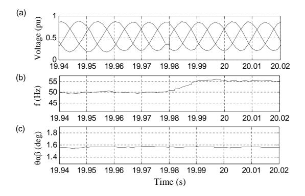
Figure 4.17: Experimental EO-PLL tracking changes in frequency from 50-55 Hz: a) Generated 3-phase voltage, b) estimated frequency, c) estimated phase
