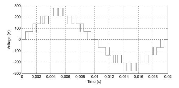
Figure 3.8: Phase Voltage of the FC-MMC under PD-PWM
