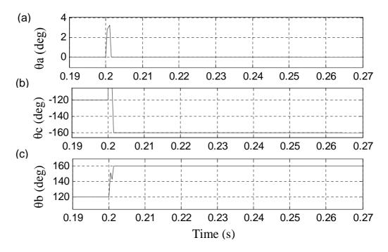
Figure 4.12: EO-PLL Estimation of Phase Angles under type C fault; (a) Phase A (degrees) (b) Phase C (degrees), (c) Phase B (degrees)
