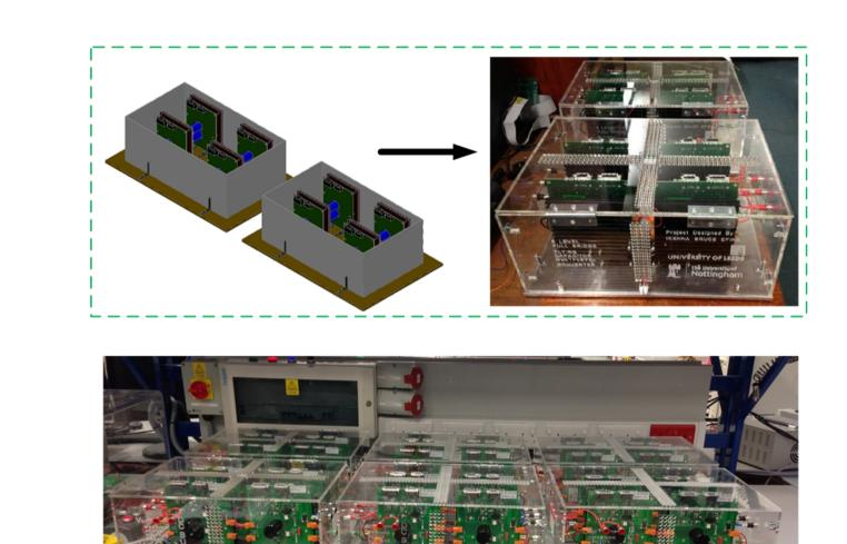
Figure 6.4: (a) Single Phase 5-level MMC-FC, (b) Three-Phase 5-level MMC-FC
