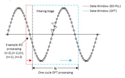
Figure 4.6: Data processing stages with a DFT as a filter
