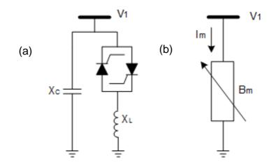
Figure 1.3: Static VAR Compensator: (a) TCR with fixed capacitor (b) Variable susceptance representation
