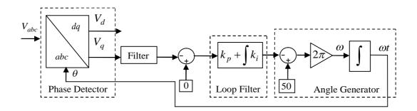
Figure 1.14: Filter +SRF-PLL
