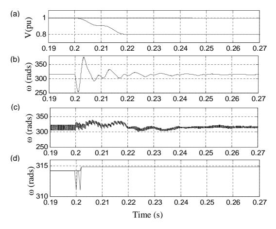
Figure 4.9: Comparison of response times for frequency tracking under type B fault (a) Peak Voltage (pu) (b) DDSRF-PLL, (c) CDSC-PLL, (d) EO-PLL
