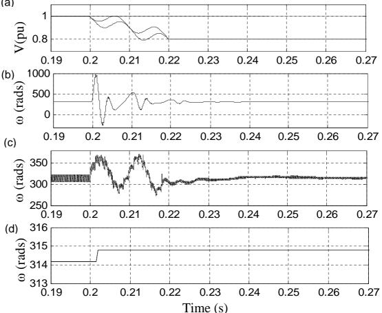
Figure 4.11: Comparison of response times of schemes for angular frequency tracking under type C fault (a) Peak Voltage (pu) (b) DDSRF-PLL, (c) CDSC-PLL, (d) EO-PLL
