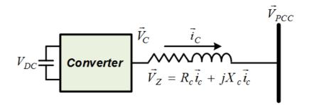
Figure 5.5: Voltage-Current relationship between Converter and PCC
