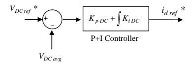
Figure 5.12: Capacitor DC Voltage Controller
