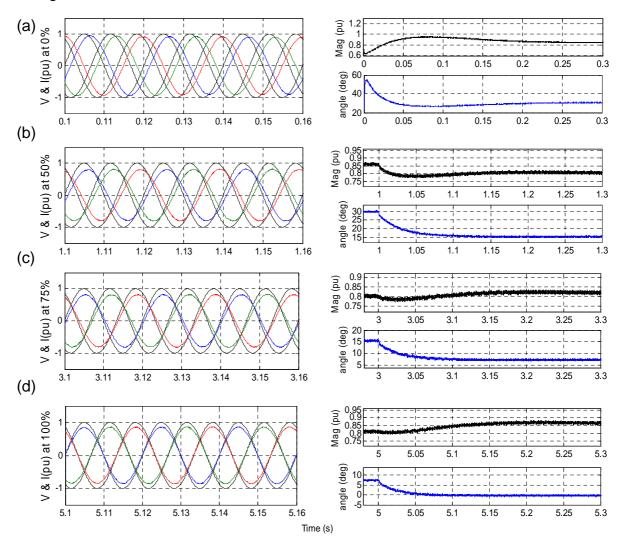
Figure 5.21: Voltage, Current and Power Factor Angle, (a) no compensation, (b) 50% compensation, (c) 75% compensation, (d) 100% compensation
