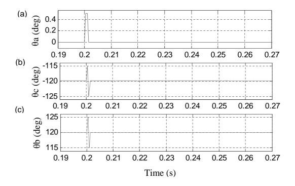
Figure 4.10: EO-PLL Estimation of Phase Angles under type B fault; (a) Phase A (degrees) (b) Phase C (degrees), (c) Phase B (degrees)
