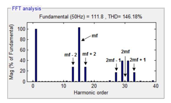
Figure 3.3: Total Harmonic Distortion (THD) for Bipolar Switching
