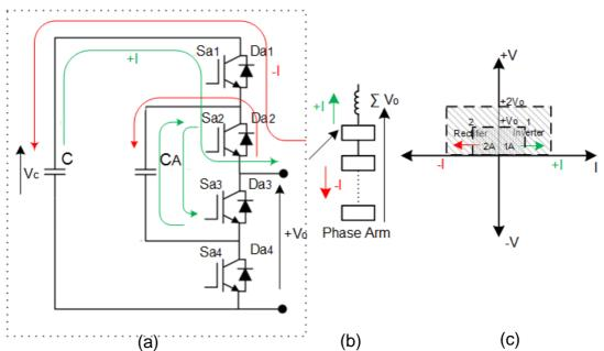
Figure 2.7: FC Half-bridge Sub-module: (a) Power Circuit showing Rectifier and Inverter Modes (b) Sub-module arrangement for one phase (c) I-V two Quadrant operations
