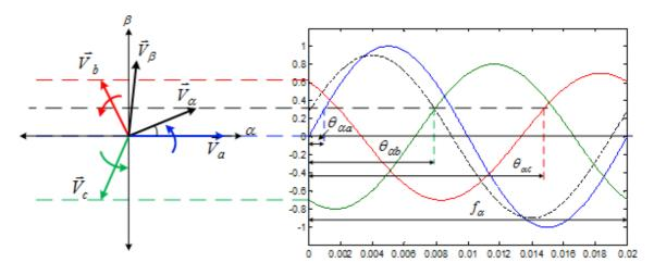
Figure 4.5: Graphical Illustration of EO-PLL Under Unbalanced Voltages
