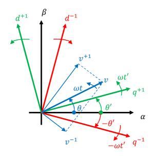
Double Synchronous Reference Frame (DDSRF)
