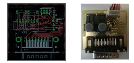
Figure 6.9: Fibre Optic Receivers PCB Design
