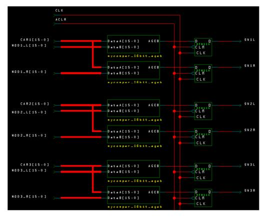
Figure 6.32: Pulse Generation unit in FPGA
