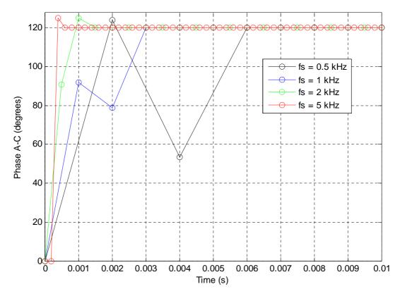
Figure 4.3: Phase angle estimation of a voltage signal at different sampling frequencies
