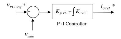
Figure 5.13: PCC Voltage Controller
