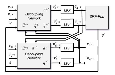
Decoupling Network + SRF-PLL (DDSRF-PLL)
