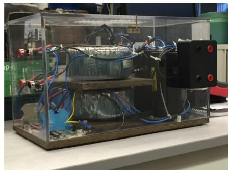
Figure 6.16: Built Isolated DC Power Supply (One Phase)
