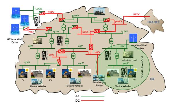
Figure 1.1: Future Transmission and Distribution Grid System
