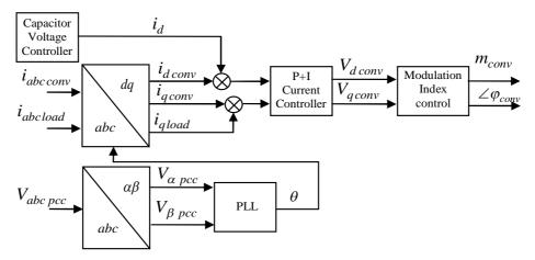
Figure 7.3: Block Diagram of the Control System
