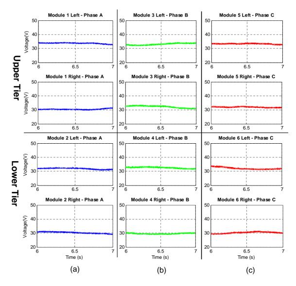
Figure 7.22: Inner Capacitor Waveforms
