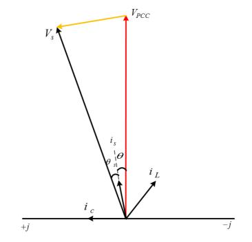
Figure 5.3: Phasor Diagram showing  $|V_S| = |V_{PCC}|$  operation
