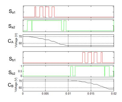
Figure 3.11: PD-PWM Switching actions for One sub-module in a fundamental cycle
