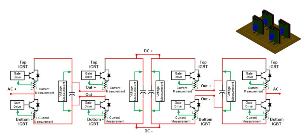
Figure 6.3: 5-level Full bridge Flying Capacitor
