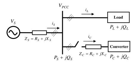
Figure 5.1: Single Line Diagram of Power System
