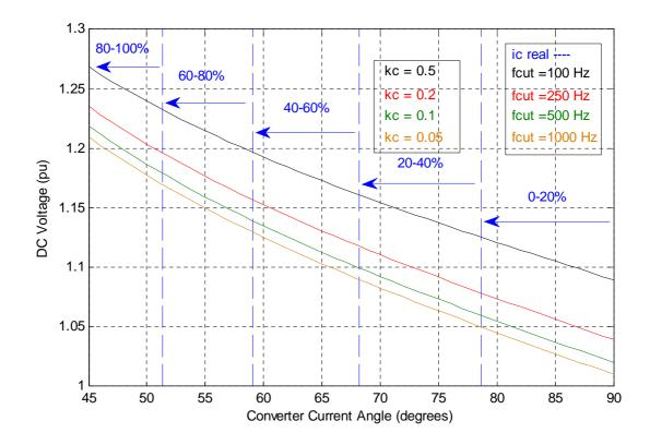
Figure 5.8: Changes in Converter Current phase Angle Vs Required DC Voltage when  $k_f = 0.4$  for fc between 100Hz to 1kHz.
