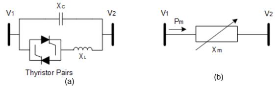
Figure 1.2: Thyristor Controlled Series Capacitor: (a) Thyristor Controlled Reactor with fixed capacitor (b) Variable reactance representation
