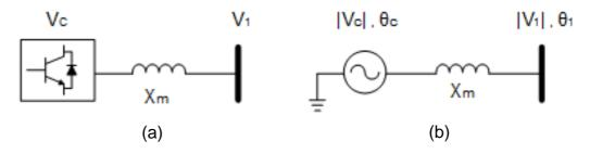
Figure 1.5: Static Synchronous Compensator: (a) Converter shunt connected to the network (b) Equivalent power circuit representation
