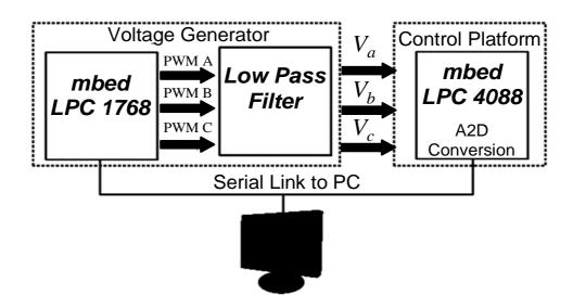
Figure 4.14: EO-PLL hardware test circuit setup
