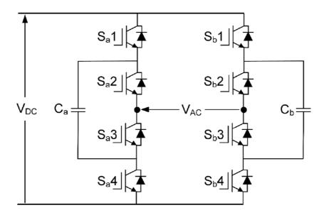
Figure 1.8: H-bridge configuration of a five-level Flying Capacitor Multilevel Inverter
