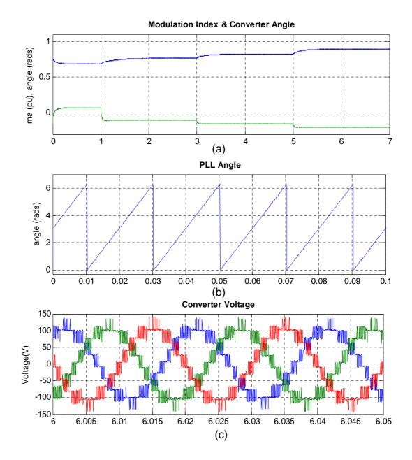
Figure 7.12: (a)Converter Modulation Index and Angle, (b) PLL Angle, (c) Converter Voltages Full Compensation
