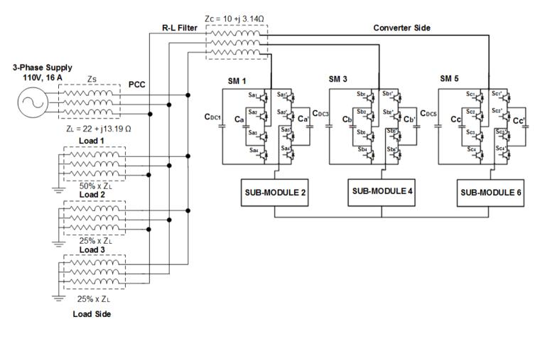
Figure 5.10: Simulation Power System Configuration
