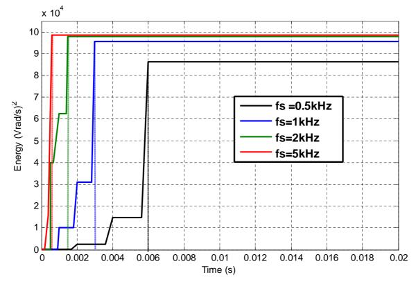
Figure 4.1: Energy of voltage signal at different sampling frequencies
