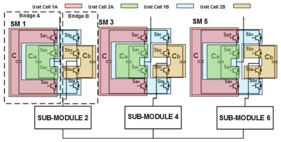
Figure 3.1: Circuit diagram of sub-modules in star configuration
