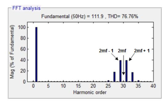
Figure 3.5: Total Harmonic Distortion (THD) for Unipolar Switching
