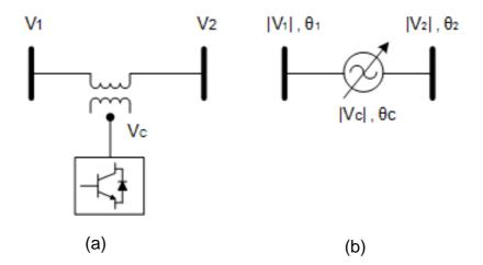
Figure 1.4: Static Synchronous Series Compensator: (a) Converter connected to network by series transformer (b) Equivalent power circuit representation
