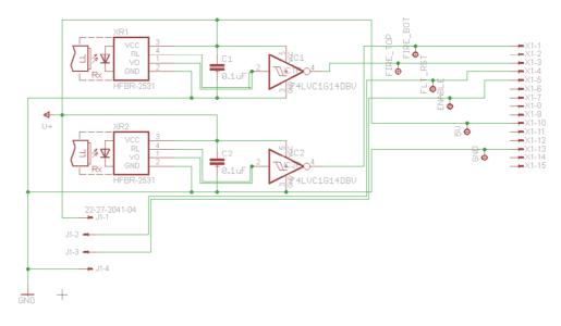
Figure 6.11: Schematic for Fibre Optic Transmitter and Receiver
