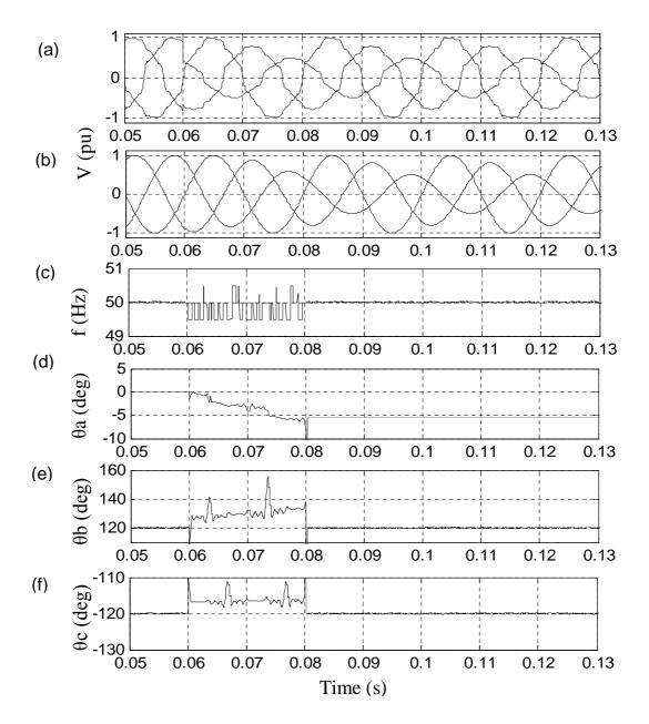
Figure 4.13: (a) Voltage with harmonics, (b) Voltage after DFT, (c) frequency detection, (d) -(f) Phase detection (A,B,C)
