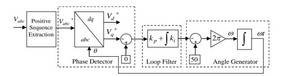
Figure 1.15: Positive Sequence Extraction + (SRF-PLL)
