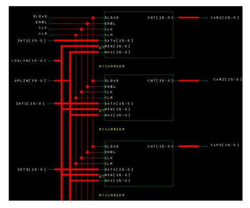
Figure 6.31: Carrier Generation Unit in FPGA
