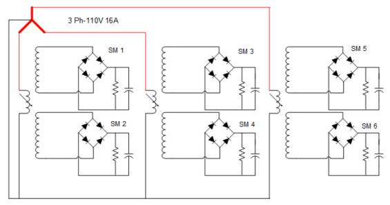
Figure 6.15: Isolated DC Power Supply Circuit
