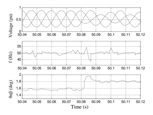
Figure 4.20: Detected result for 50% and 80% reduction in phase-B and phase-C respectively amplitude with no pre-filtering: a) Generated 3-phase voltage, b) estimated frequency, c) estimated phase
