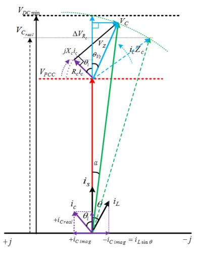
Figure 5.6: Phasor Diagram between Converter and PCC voltages & currents
