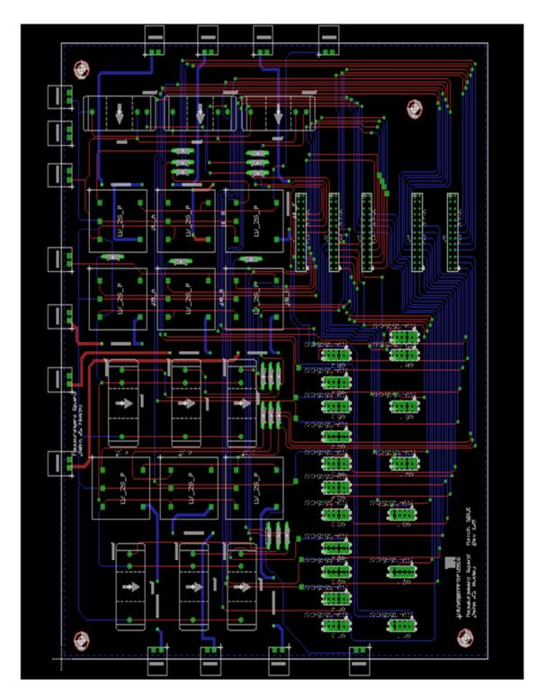
Figure 6.22: PCB Schematic for PCC Measurement Box
