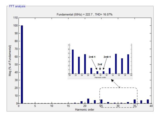
Figure 3.9: Phase voltage spectrum & THD value for PD-PWM at  $m_f$  =15
