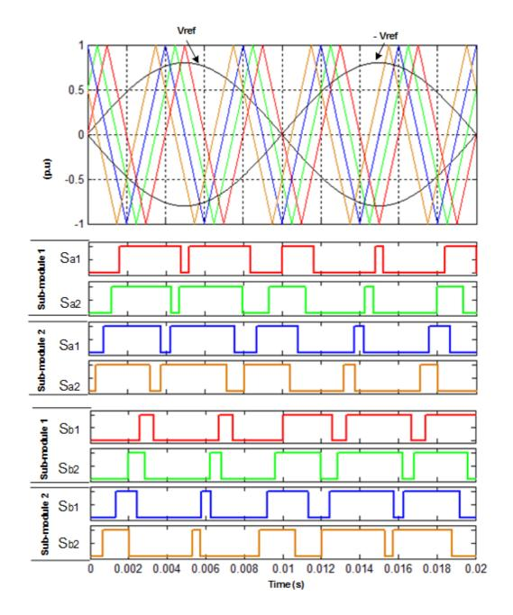
Figure 3.12:Phase Disposition PWM applied to FC-MMC at  $m_f = 5$
