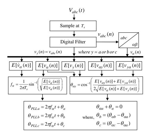
Figure 4.4: Block Diagram of EO-PLL Implementation
