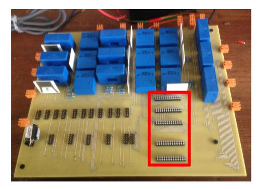
Figure 6.19: Populated PCB of PCC Measurement Box
