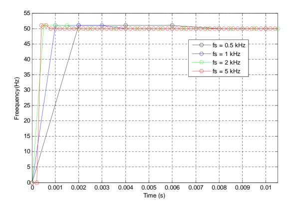
Figure 4.2: Frequency estimates of voltage signal at different sampling frequencies
