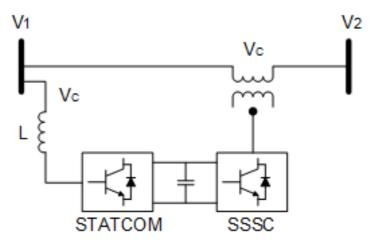
Figure 1.6: Unified Power Flow Controller
