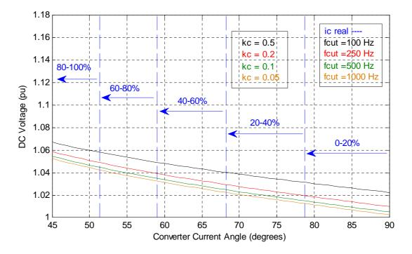
Figure 5.9: Changes in Converter's Current Angle Vs Required DC Voltage when  $k_f = 0.1$  for fc 100Hz – 1kHz.
