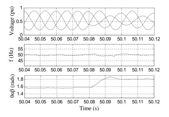
Figure 4.19: Detected result for 50% and 80% reduction in phase-B and phase-C respectively amplitude: a) Generated 3-phase voltage, b) estimated frequency, c) estimated phase
