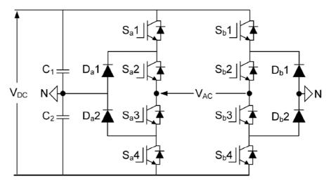
Figure 1.7: H-bridge Configuration of a Neutral Point Clamped Converter
