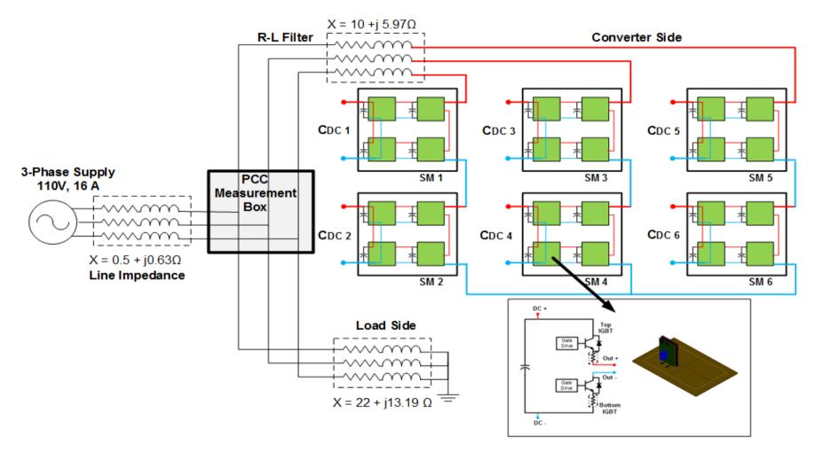
Figure 7.1: Experimental Power System Configuration
