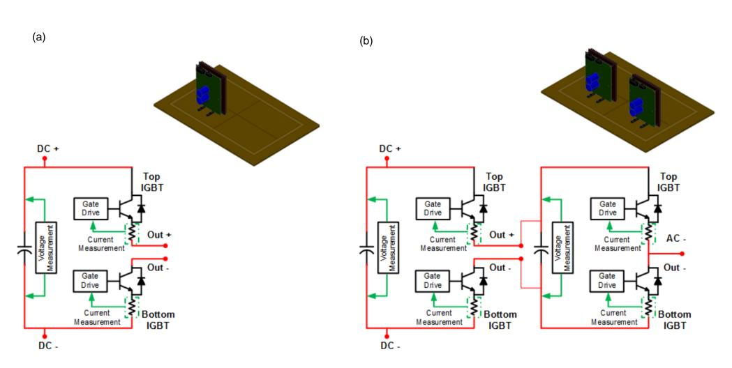
Figure 6.2: (a) Unit Power Cell (Half-bridge), (b) 5-level Half-bridge Flying Capacitor
