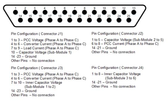
Figure 6.24: Pin Layout for Breakout Connectors
