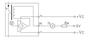
Figure 6.18: Current Transducer Circuit
