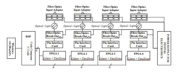
Figure 6.25: Block Diagram Software Control Unit
