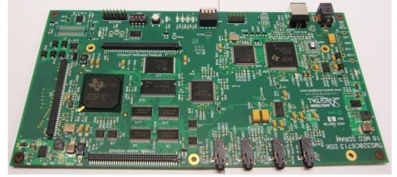
Figure 6.33: Texas Instrument TMS320C6713 DSP
