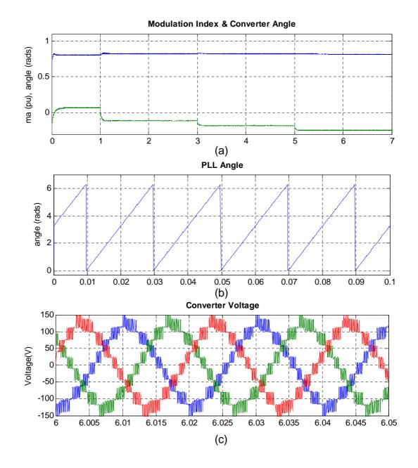
Figure 7.20: (a)Converter Modulation Index and Angle, (b) PLL Angle, (c) Converter Voltages Full Compensation
