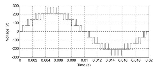
Figure 3.13: Phase Voltage of the FC-MMC under PS-PWM
