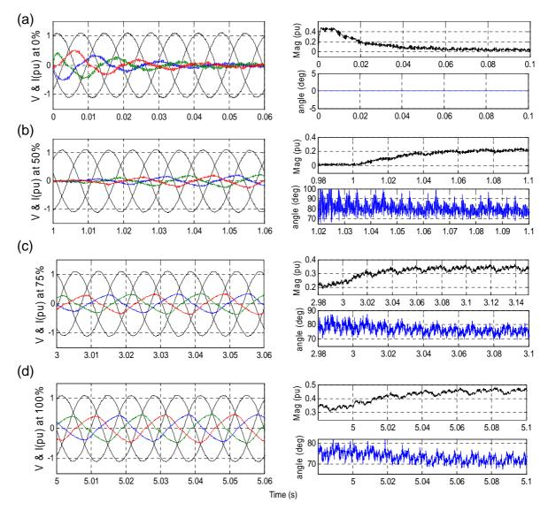
Figure 7.19: Voltage, Current and Converter Angle, (a) Zero compensation, (b) 50% compensation, (c) 75% compensation, (d) Full compensation
