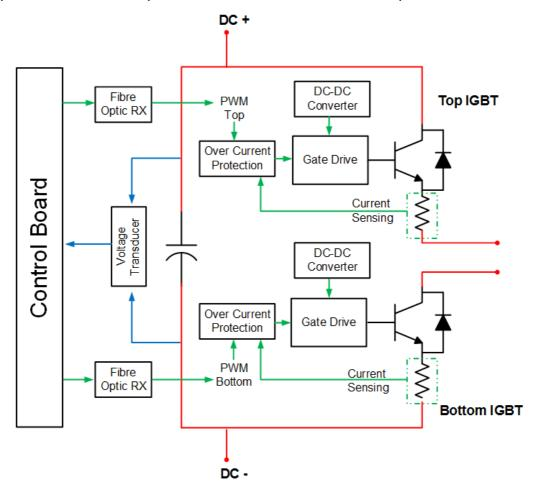
Figure 6.5: Unit Power Cell Circuit Diagram
