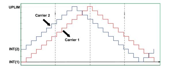
Figure 6.30: Triangular Carrier Generation
