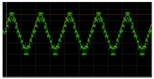
Figure 7.4: Synchronised Voltage (One Phase)
