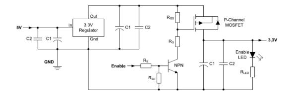
Figure 6.13: +3.3 V Switch Mode Power Supply
