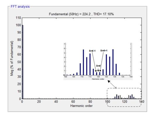
Figure 3.14: Phase Voltage Spectrum & THD value for PS-PWM at  $m_f$  =15
