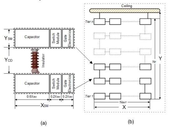
Figure 2.2: Guideline for Footprint Assessment (a) Sub-module Footprint with insulator (b) Platform Footprint with sub-modules
