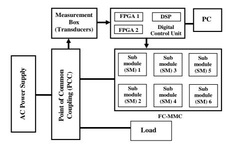
Figure 6.1: Block Diagram of FC-MMC STATCOM
