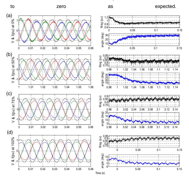
Figure 7.18: Voltage, Current and Power Factor Angle, (a) Zero compensation, (b) 50% compensation, (c) 75% compensation, (d) Full compensation
