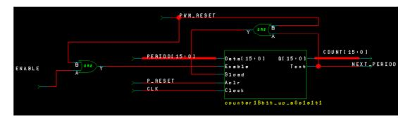
Figure 6.29: 16-bit Interrupt Counter
