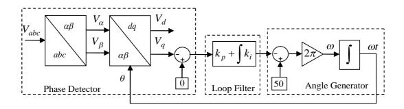
Figure 1.13: Synchronous Reference Frame PLL (SRF-PLL)
