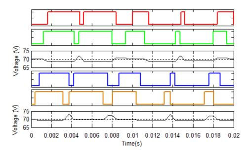
Figure 3.16: PS-PWM Switching actions in a fundamental cycle
