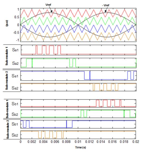
Figure 3.7: Phase Disposition PWM applied to FC-MMC at  $m_f = 15$
