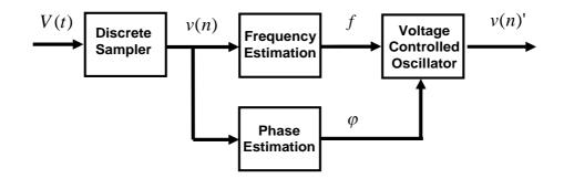
Figure 1.11: Basic structure of an open loop synchronisation technique
