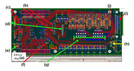
Figure 6.26: Actel Pro Asic 3 FPGA Layout
