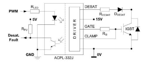
Figure 6.8: Gate Drive Circuit
