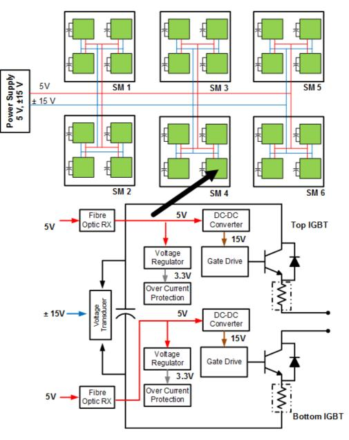
Figure 6.12: Power Supply Layout
