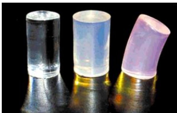
Figure 1.19: Left: pure polystyrene polymer cylinder; middle: hard polymer material containing both polystyrene and a LMWG network; right rubbery polymer containing both poly(2-ethyl hexyl methacrylate) and a LMWG network. Image reproduced from reference 64.
