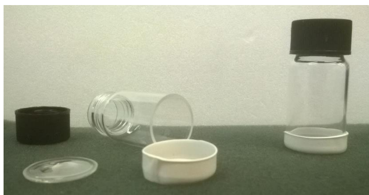
Figure 2.15: Vials used in the preparation of some hydrogel samples for rheological analysis; left: disassembled vial; right: reassemble vial, where removable base is held in place with the heat-shrink seal.
