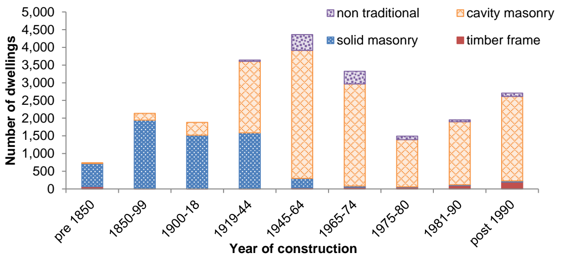
Figure. C-3 House wall types by year of construction for UK houses taken from (DCLG, 2010)
