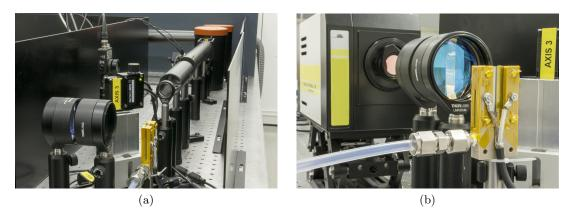
Figure 3.5: Photographs of (a) beamline with attenuation stage, photodiode pulse energy detection stage, and APPJ. (b) shows the APPJ mounted vertically on the 3-axis motorised stage, detection optics, and iCCD with filter.
