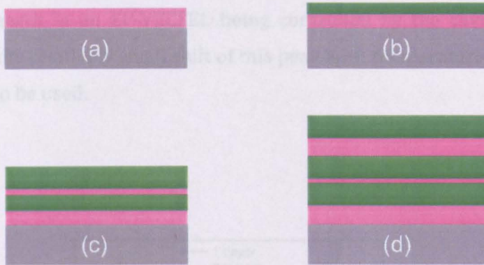
Figure 2.5 Schematic of different anti-reflective layer coating designs (a) single layer (b) dual layer (c) four layer (d) six layer
